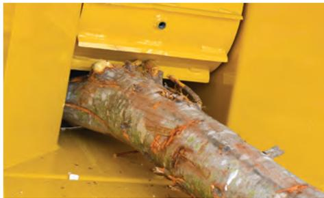
**LARGE RECTANGULAR FEED OPENING.** The large feed opening helps boost productivity by reducing the need to trim heavily branched material before feeding it into the chipper.
