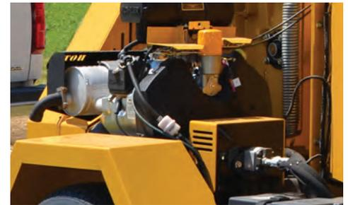
**37 HP (27.6 KW) GAS ENGINE.** The BC900XL is equipped with a Kohler Command CH1000 gas engine with no-spill oil filter change, providing 37 hp (27.6 kW) to process branches and ease of serviceability.
