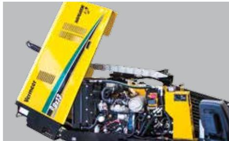
**SERVICEABILITY.** A one-piece, hinged hood offers durability as well as easy access to key service points.
