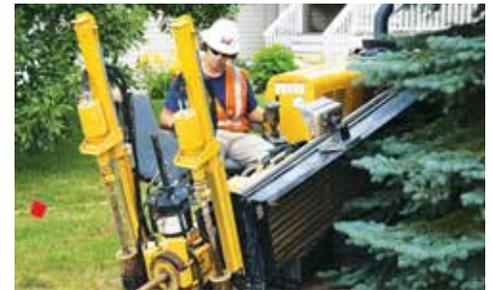
**NARROW WHEN NEEDED.** With a slender profile, the D9x13 S3 can easily maneuver within narrow jobsites and yard gates. To enhance sidehill stability and ease loading and unloading, the tracks extend 6.5" (16.5 cm) outward, adding up to 18% more width (at the tracks).
