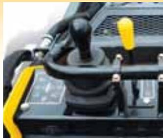
*Ground drive is controlled by a single joystick, giving the operator a smooth range of motion.*
