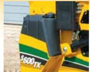
*With a 15-gal (56.8 L) fuel tank, the S600 and S600tx boast the largest tank capacity in their class, eliminating the need for refueling during the typical workday. The 14-gal (53 L) hydraulic tank is also the largest of its class, enhancing the life of the hydrostatic system by increasing dwell time of the hydraulic fluid.*
