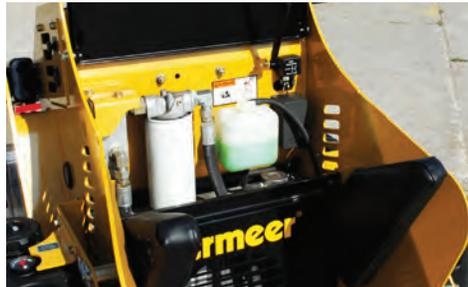
**SERVICE MADE EASY.** Pop open a panel for access to the hydraulic filter, radiator fill and electrical control board.
