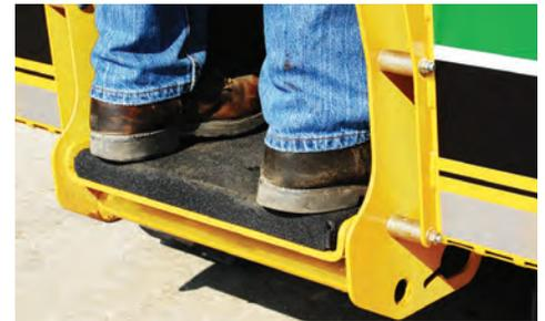
**ABOVE THE FRAY.** A dedicated, spring-cushioned platform keeps the operator out of the mud. The integrated operator presence system suspends ground drive and powered boom/bucket motion when the operator steps off the platform.
