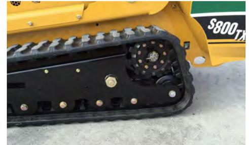
**DON'T WEAR IT OUT.** A high-mounted track sprocket eliminates wear caused by ground contact.
