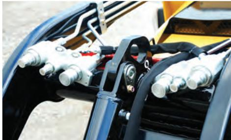
**LOW FLOW NEEDED.** An optional dual hydraulic auxiliary adds a low-flow option to the hydraulic circuit for use with dual-function attachments.
